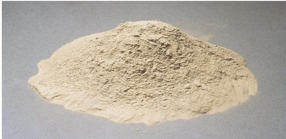
Figure 1.2 Fly ash, a powder resembling cement, has been used in concrete since the 1930s. (IMG12190) (Kapoor, Shruti, 2014).
