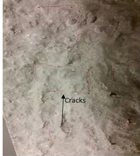
Figure 4.30b: Concrete column subject to 0% relative humidity
