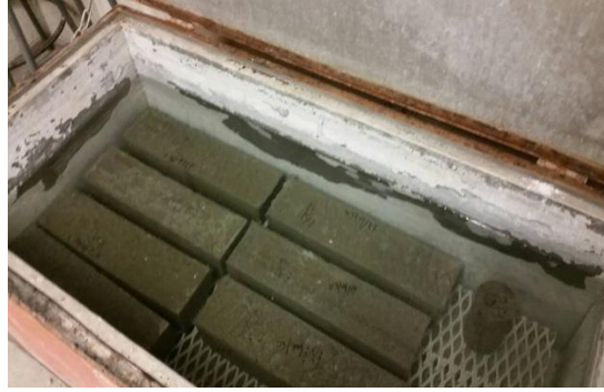
Figure 3.16: the specimens in the water tank
