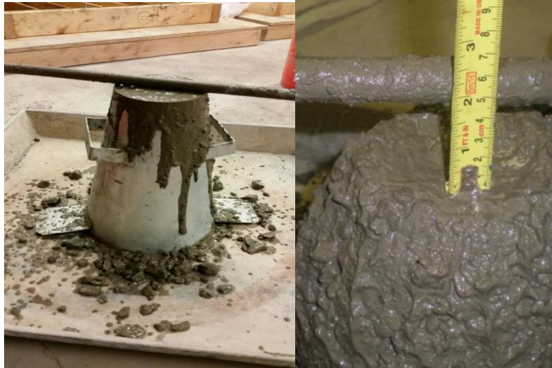
Figure 3.17a: Slump test cone filled out by concrete
