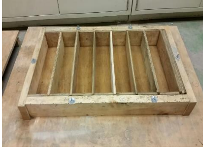
Figure 3.18a: rectangular beam molds
