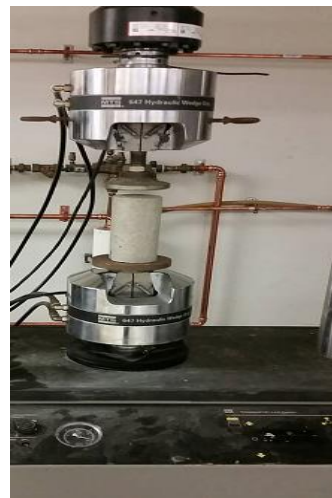
Figure 3.10b: A high capacity MTS-810 testing machine
