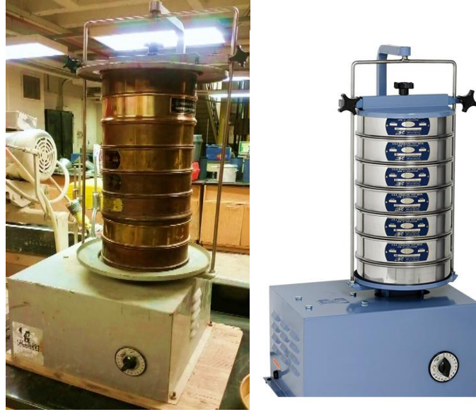
Figure 3.2: Testing sieve mechanical shaker (CA-1500, Sieve Shaker, 8" Sieves)
