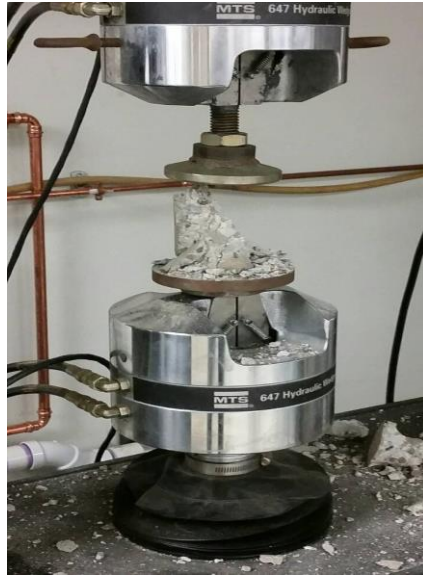
Figure 4.12: Concrete compression failure of Control specimen
