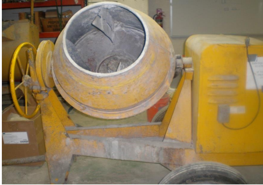
Figure 3.14: Heavy duty concrete mixer.
