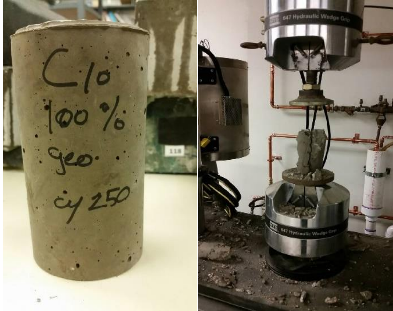
Figure 4.23: Compressive strength test for geo-polymer concrete columns
