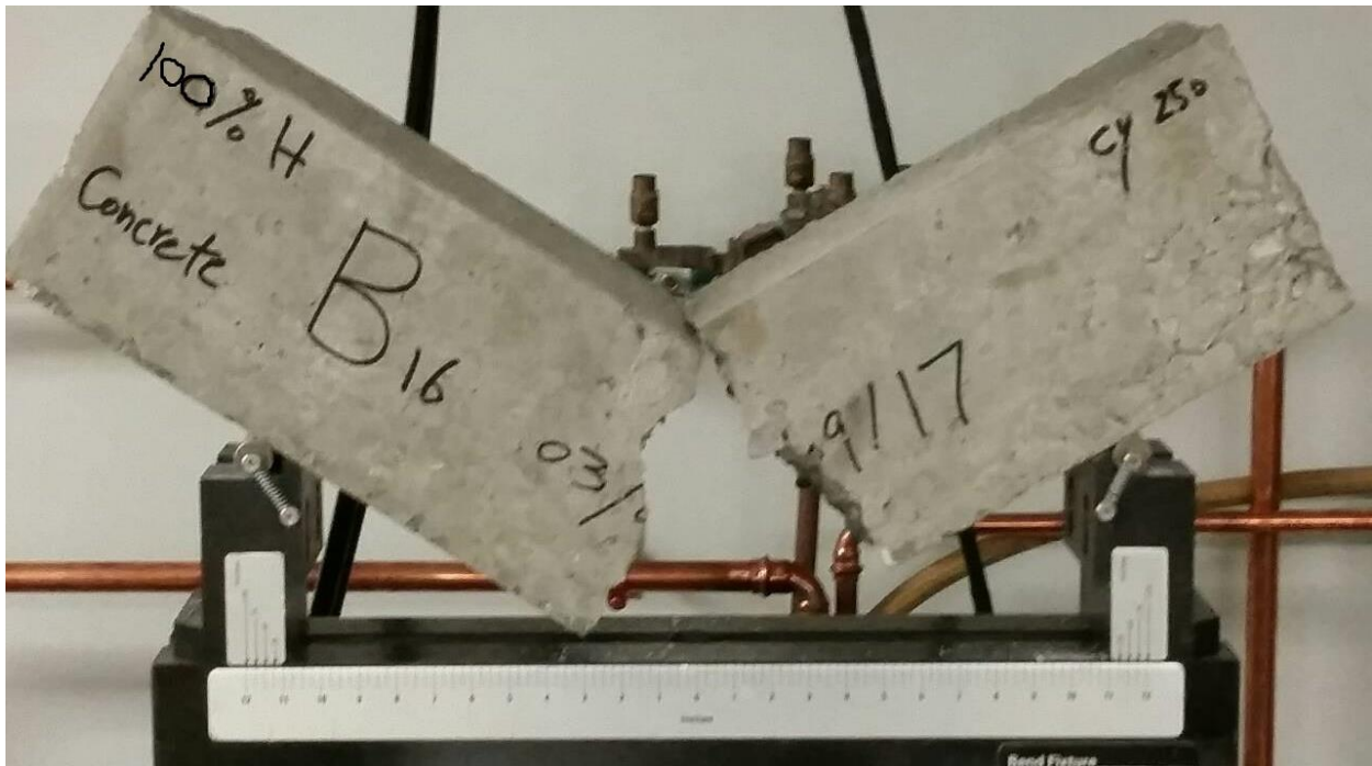
Figure 4.5: Flexural failure of concrete beam-100% relative humidity
