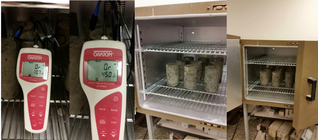
Figure 4.28: Concrete column specimens (0% relative humidity)
