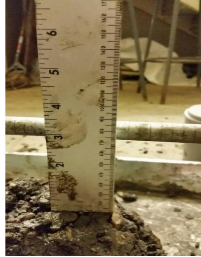
Figure 3.9d: measure the slump value (S4)
