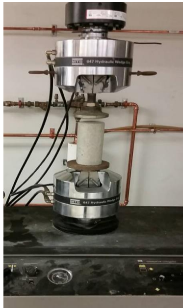
Figure 4.11: Compressive strength test “control specimen”
