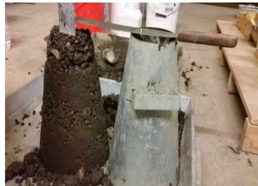
Figure 3.9b: measure the slump value (S3)
