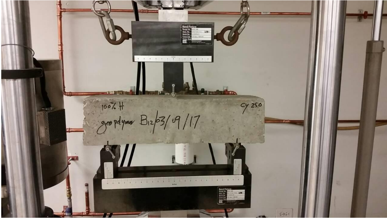
Figure 4.18a: geo-polymer Concrete beam subjected to flexural load test
