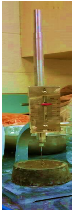
Figure 3.8: Vicat's needle for setting time test
