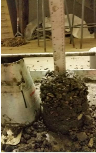
Figure 3.9c: measure the slump value (S2)
