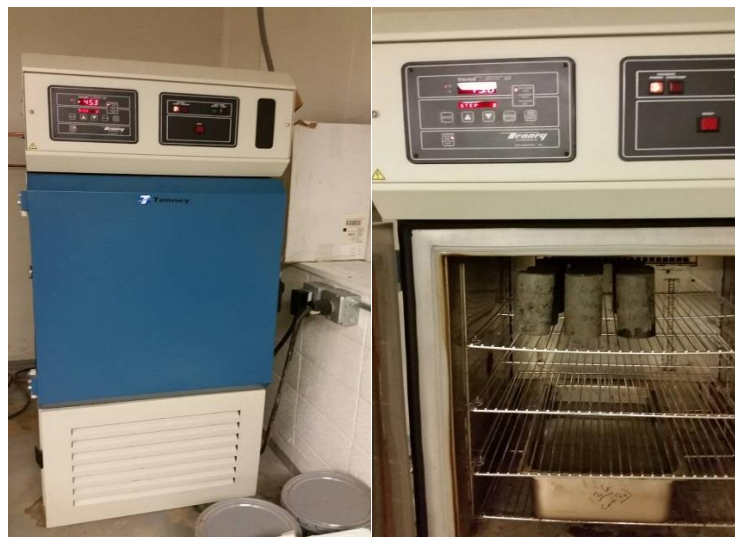
Figure 3.20: Temperature/Humidity environmental chamber
