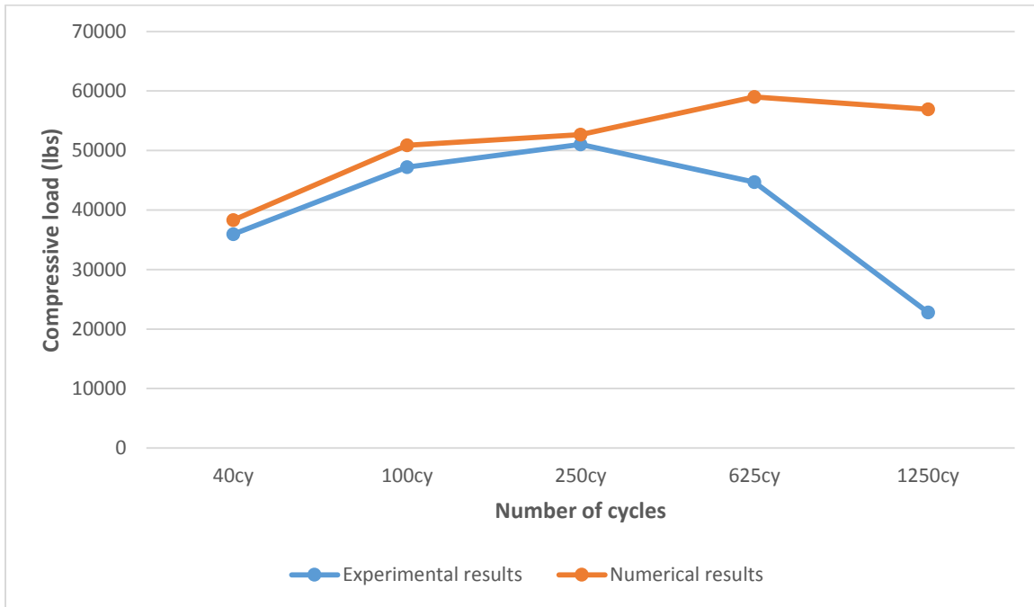
Figure 6.14: Numerical and experimental load/number of cycle curves of regular concrete column
